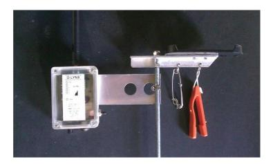
When used on round rods, the bracket can be folded in when not in use to make storing and carrying the stands easier – as shown below.
