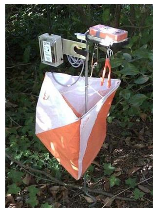
When used on round rods, the bracket can be folded in when not in use to make storing and carrying the stands easier .
