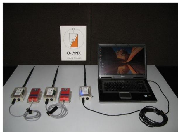
Figure 4: O-Lynx connected to a computer
