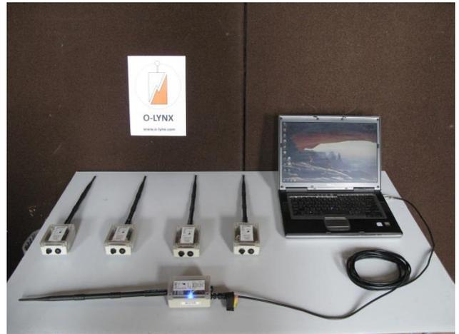
However if you are adding radios to a set or replacing the **Master** radio then the **Control** radios will need to be taught to talk to the correct **Master**. The **Master** radio can be recognised by a "MASTER" label and also has the heartbeat switch on the right side. Most Master Radios will also have red pin striping on the front Panel.
