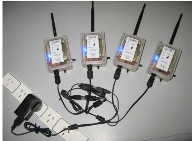
The master radios blue charging light may turn on during an event as it has been designed to charge up via the computers USB port when connected. This uses a low power charging circuit to ensure it is compatible with all USB ports.
